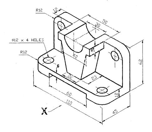
Q2 Figure given below shows the pictorial view of an object. Draw to full scale the fellowing views
