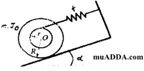
(b) One of the solution forms for free underdamped 1 d.o.f. vibration systems is given as:  $x(t) = Ae^{-\xi \phi_n t} \sin(\omega_n t + \phi)$  where displacement amplitude A and phase angle  $\varphi$  are unknown constants. Given initial disturbances in the form of displacement  $x_0$  and velocity  $v_0$ , derive the expressions for A and φ.
