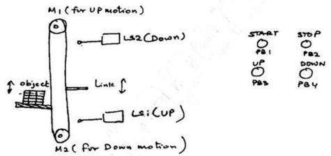
The Elevator shown in figure above employs a platform to move objects up and down. The objective is when 'UP'Button (PB3) is push the platform carries object to the up position upto LSI(Link on other side of object touches LSI), similarly when DOWN Button is pressed (PB4), the platform carries object down til LS2. M1 and M2 are separate motors used for this operation Process start with START(PBI) pressed and stops with STOP(PB2) pressed.
