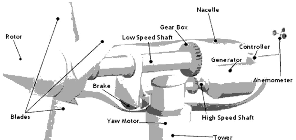
The schematic of the wind turbine components are shown here.
